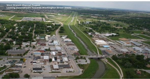
conservation will add up to an effective and comprehensive flood control effort. The improvements reduced the average annual costs of flood damages along the West Branch Papillion Creek in the protected area by at least 20 percent. The levee on top of one side of the channel also provides a route for a multi-county walking and biking trail constructed by the District from 42<sup>nd</sup> Street to Giles Road. This adds to the metro-area recreational opportunities.
